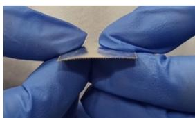
**Figure 1.** Electrode based on a 2-HEA organogel with silver deposited by sputtering.
